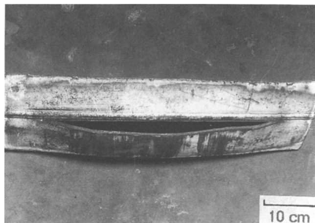
Fig. 2 Fish-mouth appearance of the rupture
